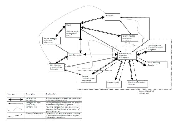
Figure 1. Supply chain map for the case study project.
