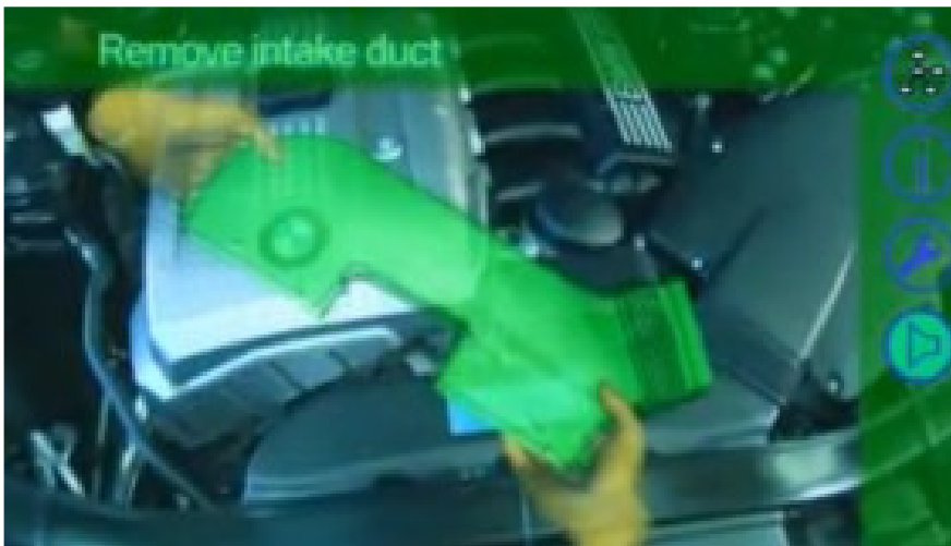
Figure 3: BMW system of cars maintenance with use of augmented reality screenshot [4].
