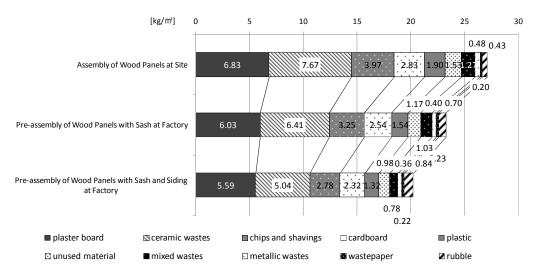
Figure 10: Comparison of industrial waste brought from construction sites
