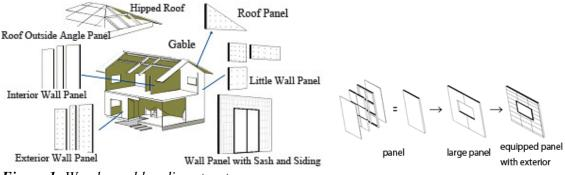
Figure 1: Wood panel bonding structure
